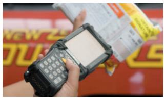
New Zealand Couriers has implemented 2D bar code scanning which allows for faster readings than conventional 1D bar codes and captures far more information.
